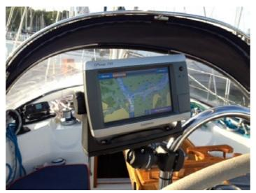
ROKK Adjustable Deck Mount on steering binnacle.
