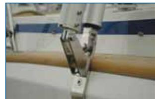
High strength base eliminates loading on backstay. Can be deck, transom or chainplate mounted.
