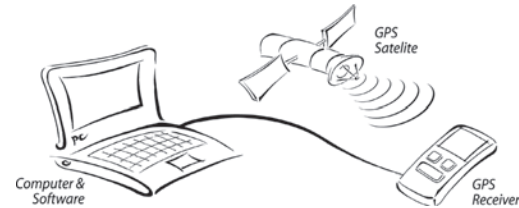
Figure 1.2 - How Navigation Systems Work
