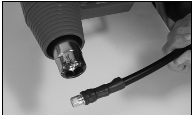
Figure 111: Applying the Heat Shrink Tubing
