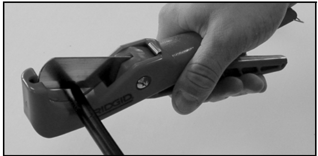
Figure 98: Cutting the Cable
