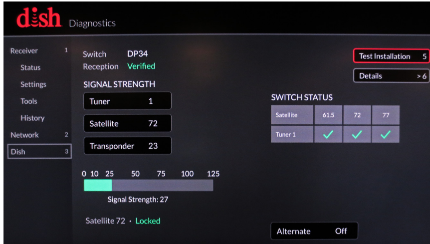
Figure 5-9 Check Switch Test Results on a Wally
