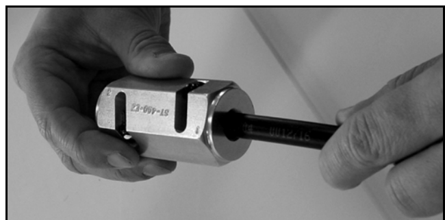
Figure 66: Stripping the End to Expose the Center Conductor
