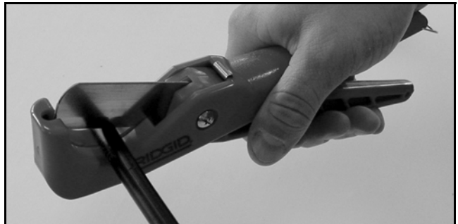
Figure 77: Cutting the Cable
