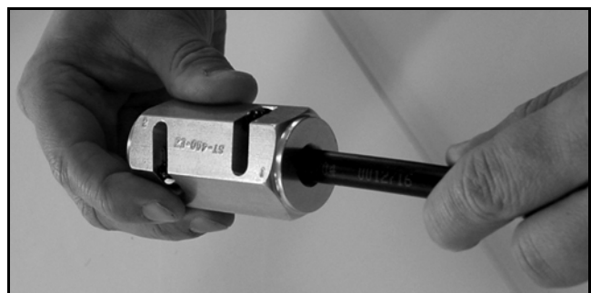
Figure 80: Stripping the End to Expose the Center Conductor
