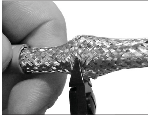
Figure 34: Cutting the Cable Braid Bulge
