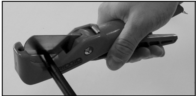
Figure 84: Cutting the Cable
