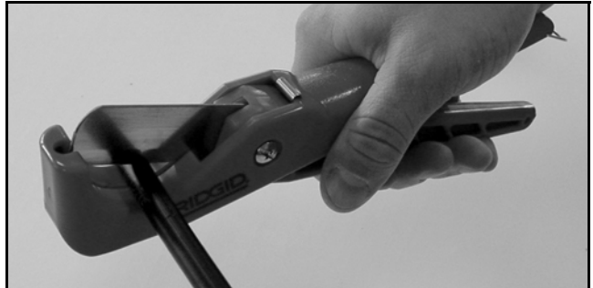
Figure 92: Cutting the Cable
