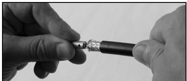
Figure 99: Deburring the Center Conductor
