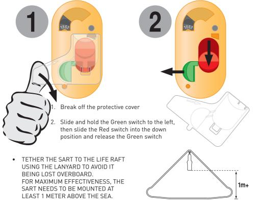
• THE SART MAY BE ATTACHED TO THE ROOF OF THE LIFE RAFT USING THE TIE PROVIDED IN THE LIFE RAFT. ALTERNATIVELY THE SART MAY BE MOUNTED ON THE TELESCOPIC POLE SUPPLIED AND ATTACHED TO THE SIDE OF THE LIFE RAFT.
