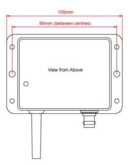
Once the unit is secured, connect the AIS/VHF antenna. Ensure the connection is fully made; should feel a slight click as the BNC locks.
