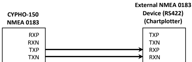
Figure 8 NMEA 0183 Connection illustration
