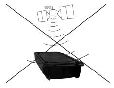
**Tip**: The label should face the sky in order to obtain the strongest GPS signal. The device should not be placed with the back cover facing the sky.
