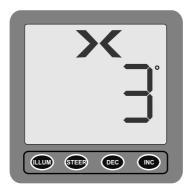
FIGURE 8 - Sensitivity Setting Display
