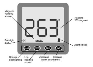
Figure 2 - Normal operation display.
