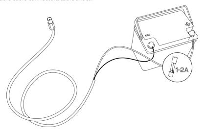
**Note:** Fuse and fuse holder are **not** included in the package.
