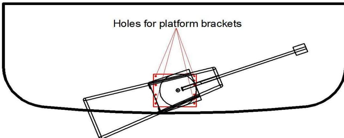
Drill the center hole and the two bolte holes for the brackets. On boats with fiber glass platform its normally not nessesary to use bolts with backing plate and nut. Drill a 6,5mm (1/4") hole, then use a 8mm (5/16) treaded tap make treads in the fiber glas. Use 8 x 20mm (5/16" x 3/4") internal hex flat-head cap screw. Use marine sealant under the mounting brackets for sealing and gluing the brackets to the platform.
