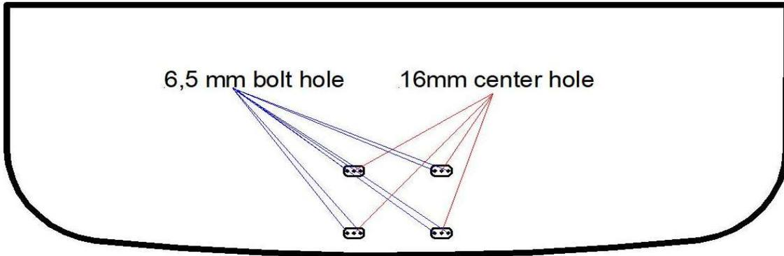
Use the four pcs 8 x 16mm internal hex flat-head cap screw and screw the bottom plate to the four mounting bracktes, use some grease on the treads. For remove the DD5 davit, unscrew the four bolts leaving just the four brackets left in the platform.
