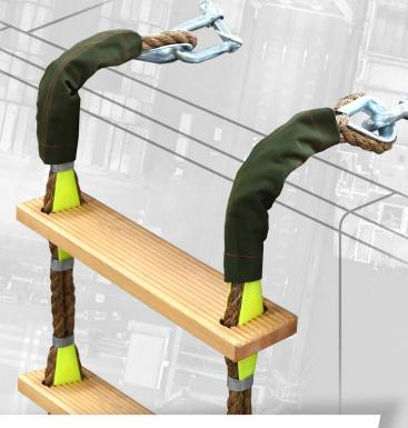
One of the most common reasons for breaking a pilot ladder is rubbing it on the ship's side. To prevent this, use rubber or wooden edge protection. Secure the section at the top of the ladder with additional protection sleeves. And check the technical condition of the rope and sleeves each time.
