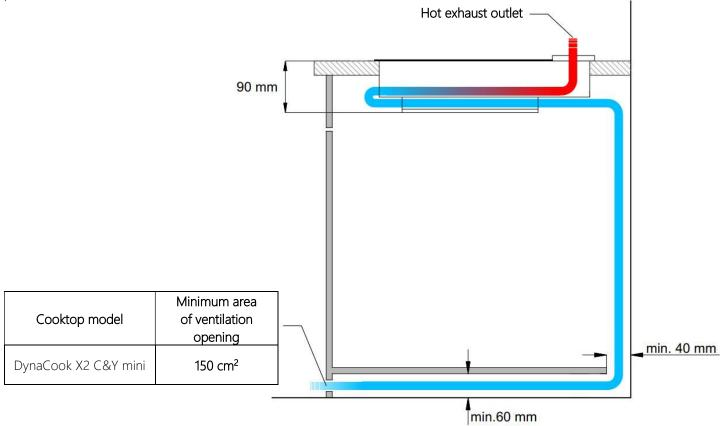
Installation in a cabinet – proper cooktop ventilation must be ensured by fulfilling the requirements specified in the figure presented below.
