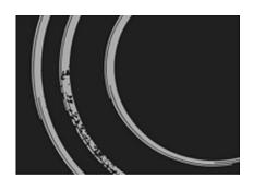
Surface decoration damaged due to application of an inappropriate cleaning agent.
