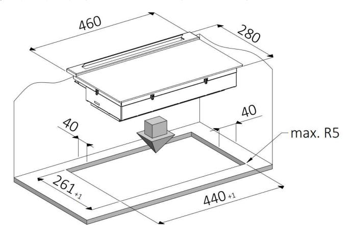
When the distance of the wall to the countertop opening is less than 40 mm, thermal insulation of the wall is required up to 200 mm from the countertop surface (ceramic material is recommended). If you should have any concerns, please contact the DynaCook Servicing Centre.
