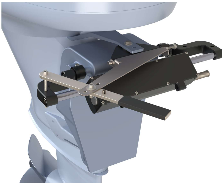
Figure 6: Emergency steering installed on steering actuator.
