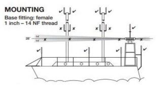
RTE Mast top –horizon +/- 25 miles. Pushpit—horizon +/- 2-3 miles. Lower installations may require trial and error to find the best location and may be subject to slight shadowing. Do not mount next to other objects as this can cause oscillation. The unit must have a clear view of the horizon.
