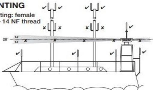
RTE Mast top -horizon +/- 25 miles. Pushpit—horizon +/- 2-3 miles. Lower installations may require trial and error to find the best location and may be subject to slight shadowing.
