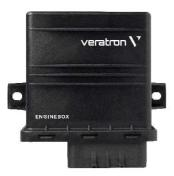
The EngineBox expands the possibilities of the NavBox for multi-engine applications or can be used as stand-alone when navigation information is not required. The EngineBox has a NMEA2000® and a J1939 CAN port. The EngineBox can also be used on older, completely analogue engines, thanks to the analogue input ports provided and designed for: RPM data, 0-400 Ohm sensors and 4-20mA sensors.
