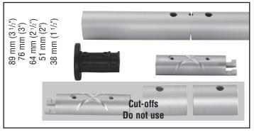
**89 – 38 mm (3** $^{1}/_{2}$ " – **1** $^{1}/_{2}$ ") Shorten top foil and adjoining full length foil so two (2) screws are used to assemble joint instead of four (4). Do not use plastic bushings above top connector.
