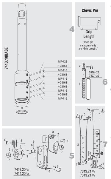
Description Order Part No. Top cover H-45412 Top cover screw (M5 X 16 mm FH) HFS1091 2 **Bottom flange** H-45413 2 Bottom flange screw (M5 X 12 mm FH) HFS1060 Guard 2 H-45562 Guard screw (M10 X 65 mm FH) 2 HFS1168 H-45264 Clamp 1 Clamp screw (M8 X 25mm FH) HFS1107 4 **Hub assembly** 1 7413.10BASE Ball plugs H-38168 5 Torlon® ball bearing (1/2") 25 MP-128 Delrin® ball bearing (1/2") MP-116 100
