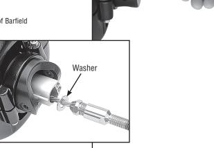
Connect eye to toggle jaw using special clevis pin. Secure using cotter pin.
