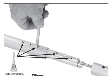
Use bushings, connector, wedge and adhesive in other screw hole and insert into other foil. Use  $1-1^{1}/_{4}$  ml of adhesive.
