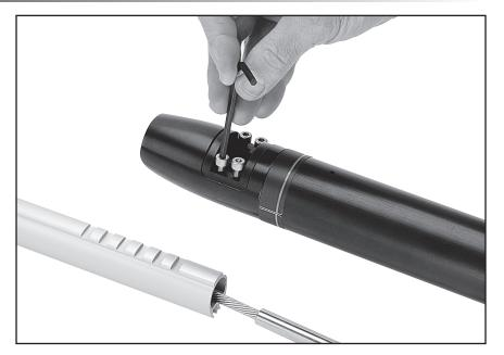
Slide drum assembly onto foils.
