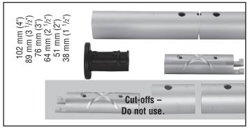
102 - 38 mm (4"  $- 1^{1/2}$ ") Shorten top foil and adjoining full length foil so two screws are used to assemble joint instead of four. Do not use plastic bushings above top connector.
