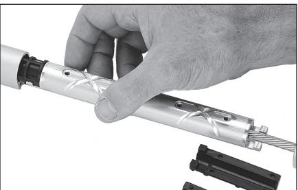
Put a drop of red Loctite  $\ensuremath{^{\circledcirc}}$  adhesive into screw holes.
