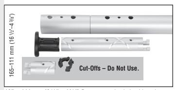
**165 – 111 mm (6** $^{1}/_{2}$ " – **4** $^{3}/_{8}$ ") Do not use plastic bushing above top connector. Cut connector right at cross formed by glue dispersion channels. Use single foil screw in top foil only.
