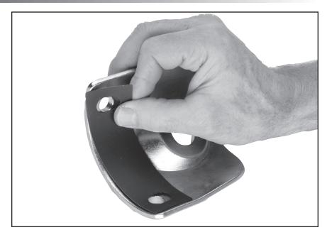
Recess turnbuckle into drum assembly, slip link plates over special clevis pin, and secure using fasteners. Use blue Loctite® adhesive on screws.
