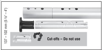
137 – 102 mm (5<sup>3</sup>/<sub>8</sub>" – 4") Do not use plastic bushing above top connector. Cut connector at cross formed by glue dispersion channels. Use single foil screw in top foil only.
