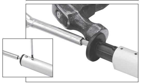
Place halves of plastic bushings on stay so hooked part of longer section faces out.
