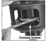
Run line through enclosed window in guard and into hole in bottom flange of spool. Tie a small overhand knot and pull it up under drum assembly.
