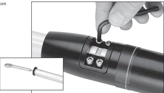
Slide halyard swivel above feeder. Place feeder in foil recess. Push screw down so tab catches under foil. Tighten screw.
