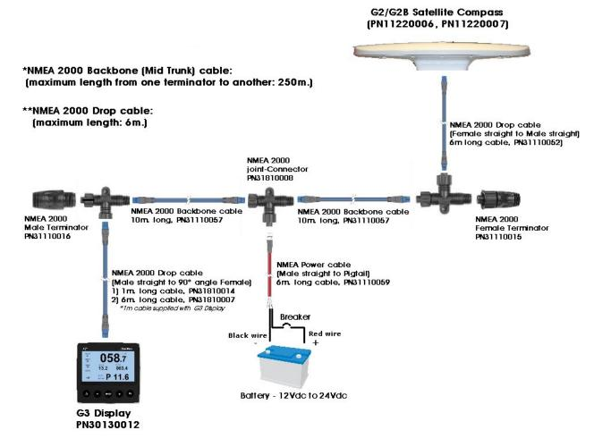
Figure 1 - Typical NMEA 2000 G2 system setup
