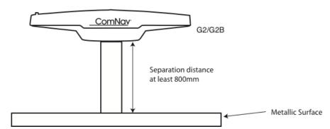
Figure 6 - Mounting distance to large metallic surface
