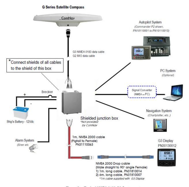
Figure 2 - Typical NMEA 0183 G2 System setup
