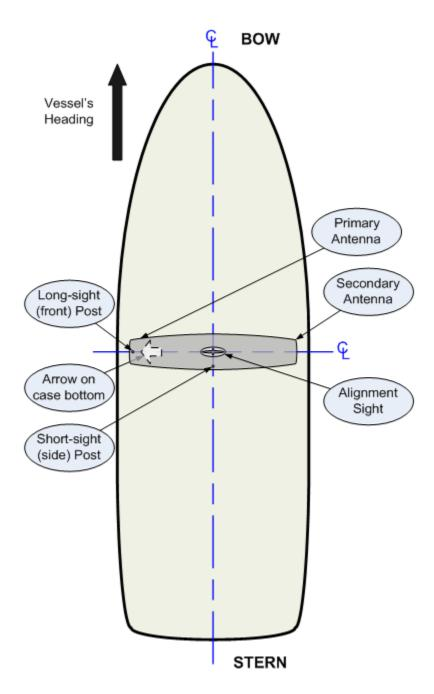
Figure 8 – Heading & Roll Installation (viewed from above). Heading bias is 90° at this orientation
