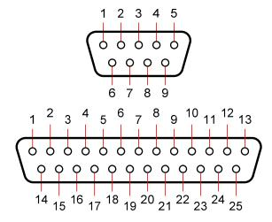
Figure 15 - DE9 & DB25 Pin Numbering
