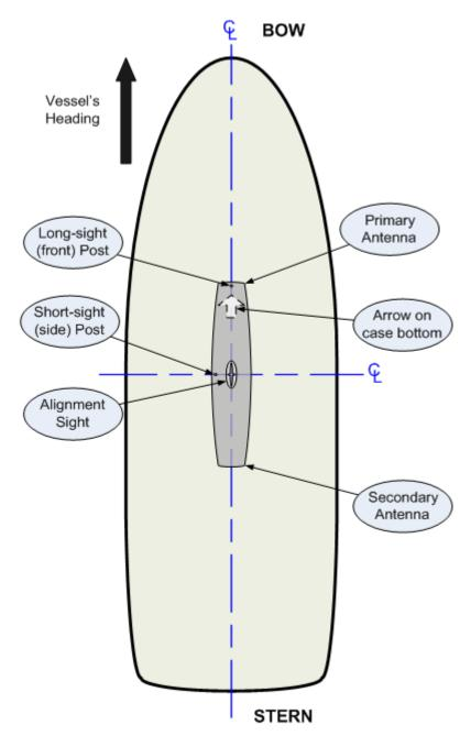
Figure 7  $\,-\,$  Heading & Pitch Installation (viewed from above). Heading bias is 0° at this orientation
