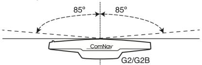
Figure 4 - Clear view required for the compass
