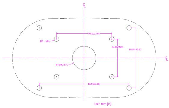
Figure 10 -Surface mount hole measurements
