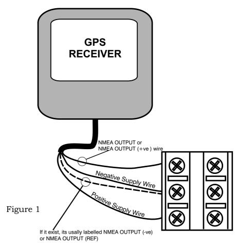
If not, then the reference is internally connected to ground, and can be ingnored
