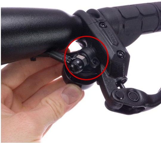
Clip the mounting bracket over the left brake lever as shown
