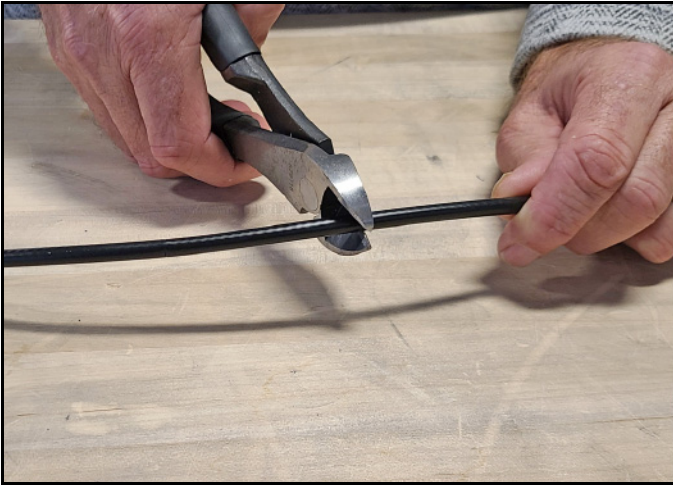
Figure 69: Cutting the Cable
