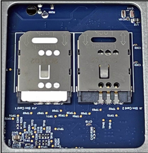
Figure 62: SIM Card Installed, Screen Locked in Place
