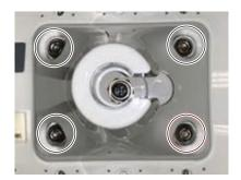
4 Verify the orientation of the HS75, then tighten the jam nut to the bottom of the pole mount bracket to a torque of 11 - 13 Nm (8 – 10 lbs-ft).
