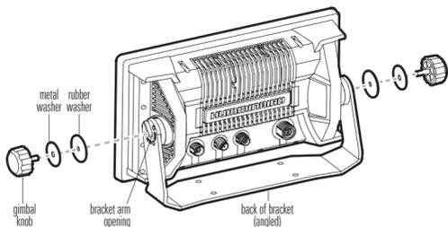
If you prefer to mount the control head overhead, flip the bracket to the top of the control head. The opening in the gimbal bracket arms must face the rear of the control head.
