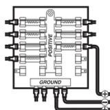
**Battery Connection:** Install an inline fuse holder (not included) and the required fuse (as shown in the **Required Fuse Size** table). Attach the black wire to ground (-), the red wire to positive (+) 12 VDC power, and the drain/shield wire to the boat's chassis ground terminal.
