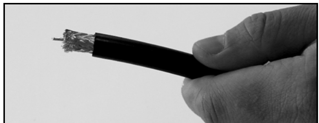
Figure 84: Cable Stripped, Exposing Dielectric
