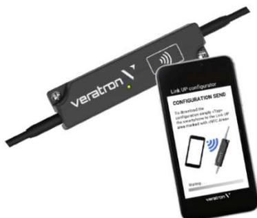
5. To download the configuration, simply “tap” the smartphone again onto the LinkUp wireless area, as described on step 1.
