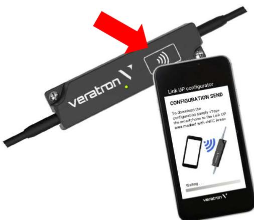
1. Launch the “Link Up Configurator” App and read the actual configuration of the LinkUp device by “tapping” the smartphone onto the LinkUp wireless area (indicated by the red arrow).
