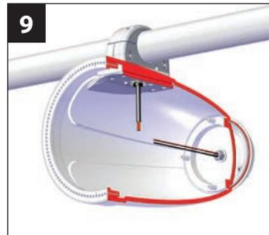
Connect the LED wires from the LED Light Cap to the LED wires entering the enclosure. Refer to the wiring charts on the opposite page for details. DO NOT install the fuse holders inside the enclosure.
