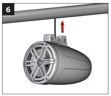
Slide the excess cable into the opening in the pipe as you raise the enclosure to flush the Lower Fixture to the pipe.
