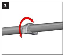
Adjust the angle of the fixture to the desired position, and mark the location for the cable hole. Remove the fixture assembly, and drill a 5/16" or 3/8" hole on the mark. If necessary, use a file or sandpaper to smooth the edges to ensure no sharp edges.
