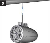
Have a helper support the enclosure during this step. Connect the 16 AWG red/stripe (+) and black/ stripe (-) speaker cable exiting the ETXv3 enclosure to the speaker cable exiting the pipe. For LED models, connect the 20 AWG blue LED (+) and yellow LED (-) as illustrated on Page 2.
