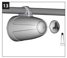
For best adhesion, it is recommended to clean the inside of the aluminum cap with acetone (not included) prior to attaching it to the enclosure. Apply a circular bead of Silicone Adhesive to the inside of the aluminum logo cap, about 1/2-inch (13 mm) from the outer edge.
