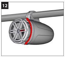
Rotate the speaker to the desired angle. Reinstall the #8 x 1-1/4" Pan Head Screws and #8 Flat Washers.
