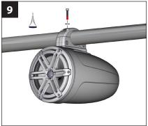
Remove one of the 1/4 - 20 x 1-1/4" Machine Screws at a time. Apply Loctite<sup>®</sup> Red Thread-Locking Compound to the screw end, reinstall, and fully tighten. Repeat the process for the other three screws.
