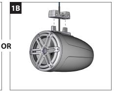
For applications where the cable can be routed through the pipe, the cable can be passed through the opening in the bottom of the Lower Fixture. Steps 2, 3, and 6 are only necessary for this option.
