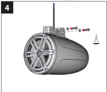
Align the Lower Fixture to the enclosure. Install (2) 5/16" Split Lock Washers and (2) 5/16 - 18 x 1-1/4" Machine Screws as pictured. Apply Loctite® Red Thread-Locking Compound to each screw end, thread them into the Lower Fixture, and fully tighten while pressing down on the Lower Fixture to ensure no gap.
