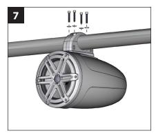
Align the two halves of the fixture around the pipe. Install (2) 1/4" Split Lock Washers and (2) 1/4 - 20 x 1-1/4" Machine Screws as pictured, and hand tighten them into the fixture. DO NOT FULLY TIGHTEN AT THIS TIME.
