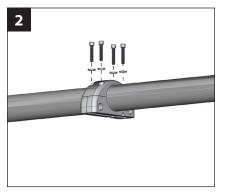
Determine the speaker mounting location. Slide a 1/4" Split Lock Washer over each of the four  $1/4 - 20 \times 1 - 1/4$ " Machine Screws, and hand tighten the screws into the Lower Fixture to temporarily secure the two fixture halves around the pipe.
