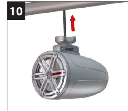
Slide the excess speaker cable and the butt connectors into the opening in the pipe as you raise the enclosure to flush the fixture to the pipe.
