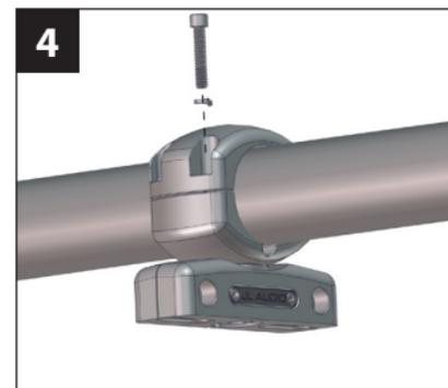
Determine the speaker mounting location, and temporarily secure the fixture around the pipe by hand tightening the four 1/4 - 20 x 1-1/4" machine screws and 1/4" lock washers.
