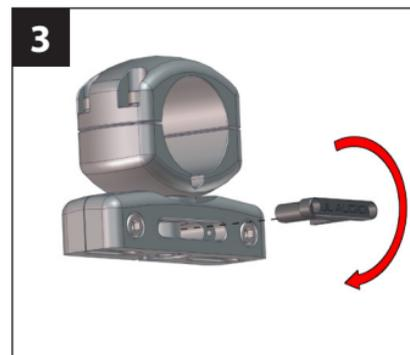
Compress the base and two upper halves of the fixture together while pushing the fork out through the small pin holes on the opposite side. Flip the fork, and reinstall, along with the two #8 - 32 x 3/8" machine screws and lock washers.
