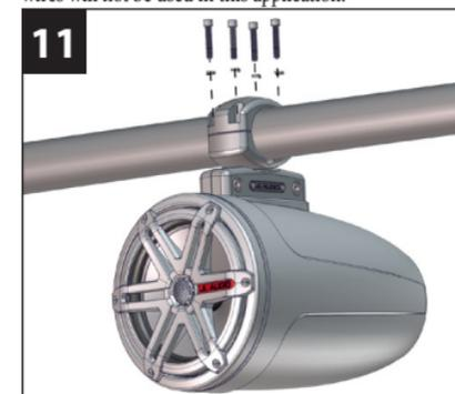
Align the two upper halves of the fixture around the pipe. Hand-tighten four 1/4 - 20 x 1-1/4" machine screws with 1/4" lock washers into the fixture. **DO NOT TIGHTEN FULLY AT THIS POINT.**
