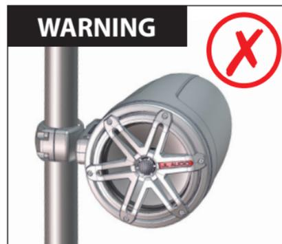
**WARNING:** Never attach swivel mounting fixtures to vertical or angled pipes.
