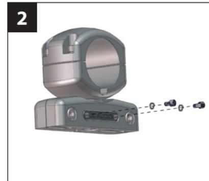
In applications that require the logo to be inverted, remove the two #8 - 32 x 3/8" machine screws and lock washers.
