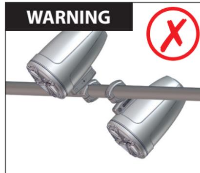
**WARNING:** Do not mount enclosures to a horizontal pipe in any position other than directly above or directly below.
