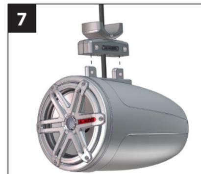
Remove the four 1/4 - 20 x 1-1/4" machine screws and 1/4" lock washers to separate the two upper halves of the fixture. Pass the speaker cable exiting the enclosure through the opening on the underside of the fixture.
