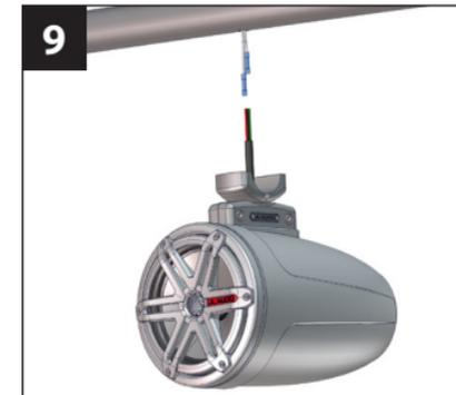
**Have a helper support the enclosure during this step.** Use the supplied butt connectors to connect the red (+) and black (-) speaker cable exiting the ETXv3 enclosure to the speaker cable exiting the pipe. The green and white wires will not be used in this application.
