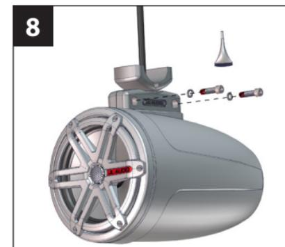
Apply Loctite® red thread-locking compound (included) to two 5/16" - 18 x 1-1/4" machine screws (included), thread them into the base of the fixture, and push down on the fixture to ensure no gap while fully tightening.
