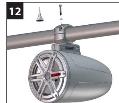
Remove one of the 1/4 - 20 x 1-1/4" machine screws and 1/4" lock washers at a time. Apply Loctite® red thread-locking compound (included), reinstall, and fully tighten. Repeat the same process for the other three screws. **(Continued on reverse.)**
