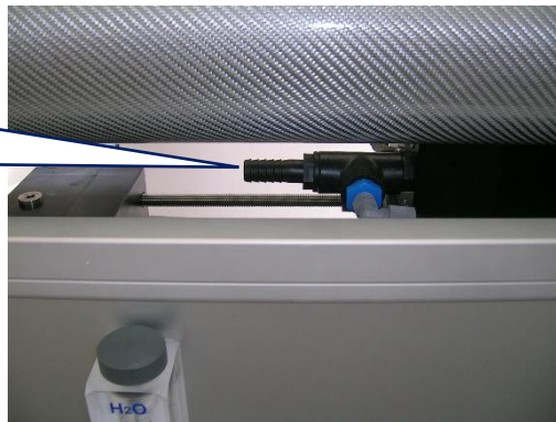
WATERMAKER INTAKE AND DISCHARGE FIG. 4-2
