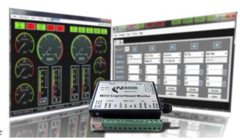
MD33 is compatible with most marine engine sensors whether or not gauges are present.
