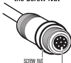
The connectors are keyed to prevent reversed installation.
