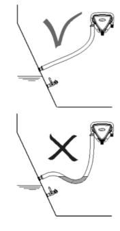
Figure 11. Water will collect in the hanging bend of the exhaust gas hose and will cause back pressure.
