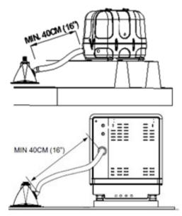
Fig 5. Waterlock min. 40cm (16") from the generator.
