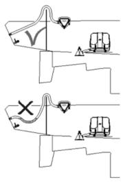
Figure 17. The gas outlet hose may go up once and then should slope down
