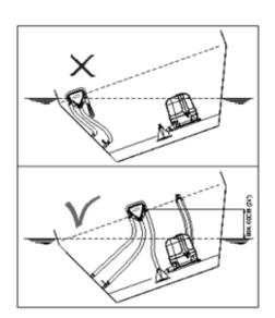
Figure 12: Siphon Breaker and Water/Gas separator min. 60cm (24") above the waterline in all circumstances.
