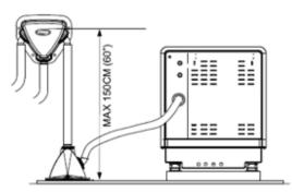
Figure 6. Maximum lift of the water/gas emulsion: 150cm (60")
