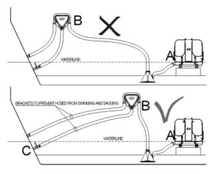
Figure 8. Keep hose between generator and Water/Gas separator as short as possible! Max. length of line between A and B is 3 meter (10'). BC may be much longer up to 7meter (21').
