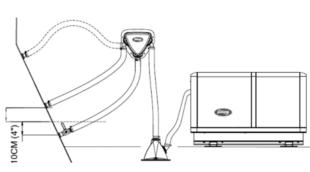
Figure 9. Water outlet max. 10cm (4") below the waterline.
