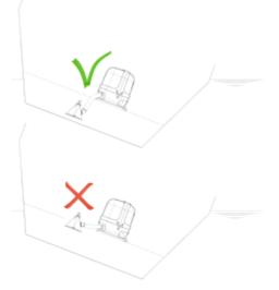
Figure 13. When heeling, the waterlock should still be below the generator to prevent water flowing back into the engine.
