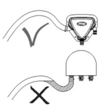
Figure 16. The WhisperPower Water/Gas separator has a higher position of the exhaust/gas outlet than most other brands.
