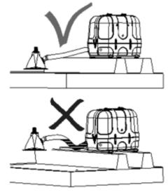
Figure 10. Let exhaust hoses from generator to waterlock run downwards only.
