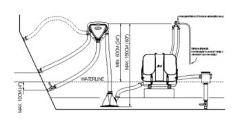
Figure. 7. Overview Water/Gas separator and Waterlock system
