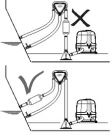
Figure 14. Place an extra muffler in the downwards sloping hose
