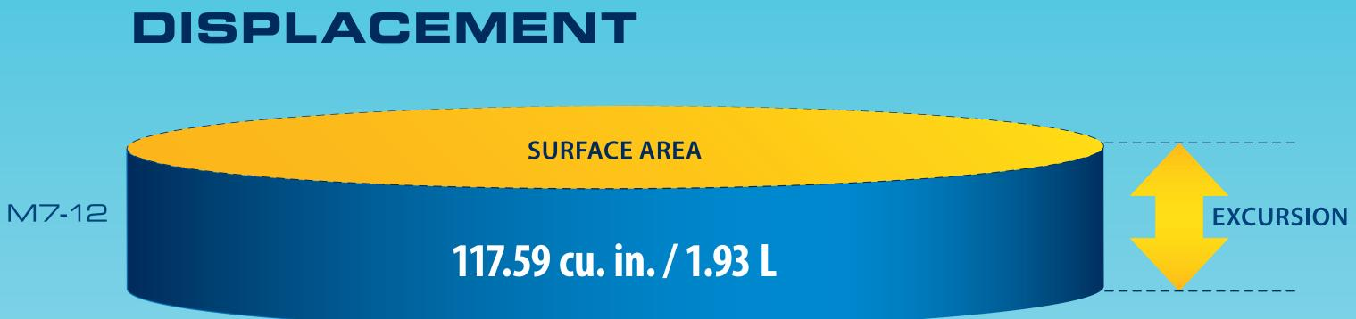
Displacement is a direct measure of a subwoofer driver's output capability. It is calculated by multiplying the moving surface area of the woofer, times its peak-to-peak linear excursion capability, much like the displacement of an engine is determined by bore x stroke.
