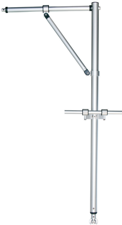
10625 Davit 1550 x 65 mm, arm 600 x 35 mm Includes NOA fittings Rope and block not included Lift capacity 20 kg
