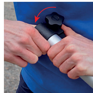
4. Twist the lock until it snap on the tube
