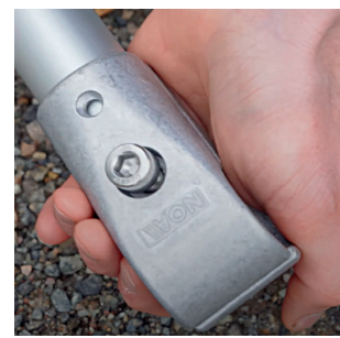
3. Put on the second half and fasten hex screw
