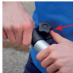
3. Use left thumb to hold lock in place
