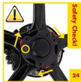
24 Ensure all three quick release levers are closed and the Hexlock™ is rotated clockwise to the locked position as shown.
