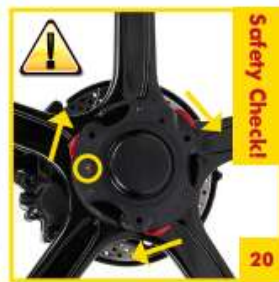
20 Ensure all three quick release levers are closed and the Hexlock™ is rotated clockwise to the locked position as shown.
