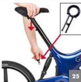
25 With the Gocycle upright, press down on the saddle and insert Lockshock pin as shown
