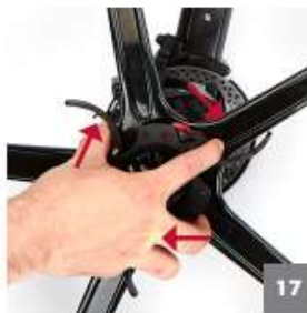
17 While holding all three cam levers fully open, mount wheel to front hub
