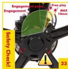
23 Open and close EACH cam lever to check that it is adjusted and operating as shown. Consult the Owner's Manual if adjustment is needed. NEVER ride with any cam "loose" or if the resistance when closing or opening is not even for all cams.
