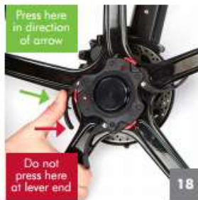
18 Close each cam lever as shown
