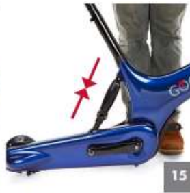
15 Continue lowering the Gocycle until the Lockshock is fully inserted
