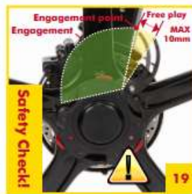
19 Open and close EACH cam lever to check that it is adjusted and operating as shown. Consult the Owner's Manual if adjustment is needed. NEVER ride with any cam "loose" or if the resistance when closing or opening is not even for all cams.
