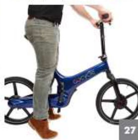
27 Recommended saddle height should allow you to touch the ground with both feet while seated
