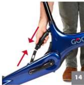
14 Align the Lockshock™ body with the Lockshock plunger as shown
