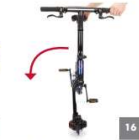
16 Rotate the pedals to the position demonstrated (right pedal up) and carefully lay the Gocycle flat
