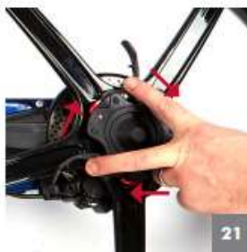
21 While holding all three cam levers fully open, mount wheel to rear hub
