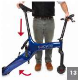
13 Carefully lower the Gocycle downwards so the Cleandrive continues to rotate backwards
