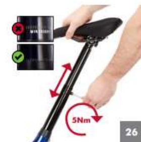
26 Select preferred saddle height. Tighten the clamp to 5Nm. (DO NOT exceed the minimum insertion mark on the seat post)
