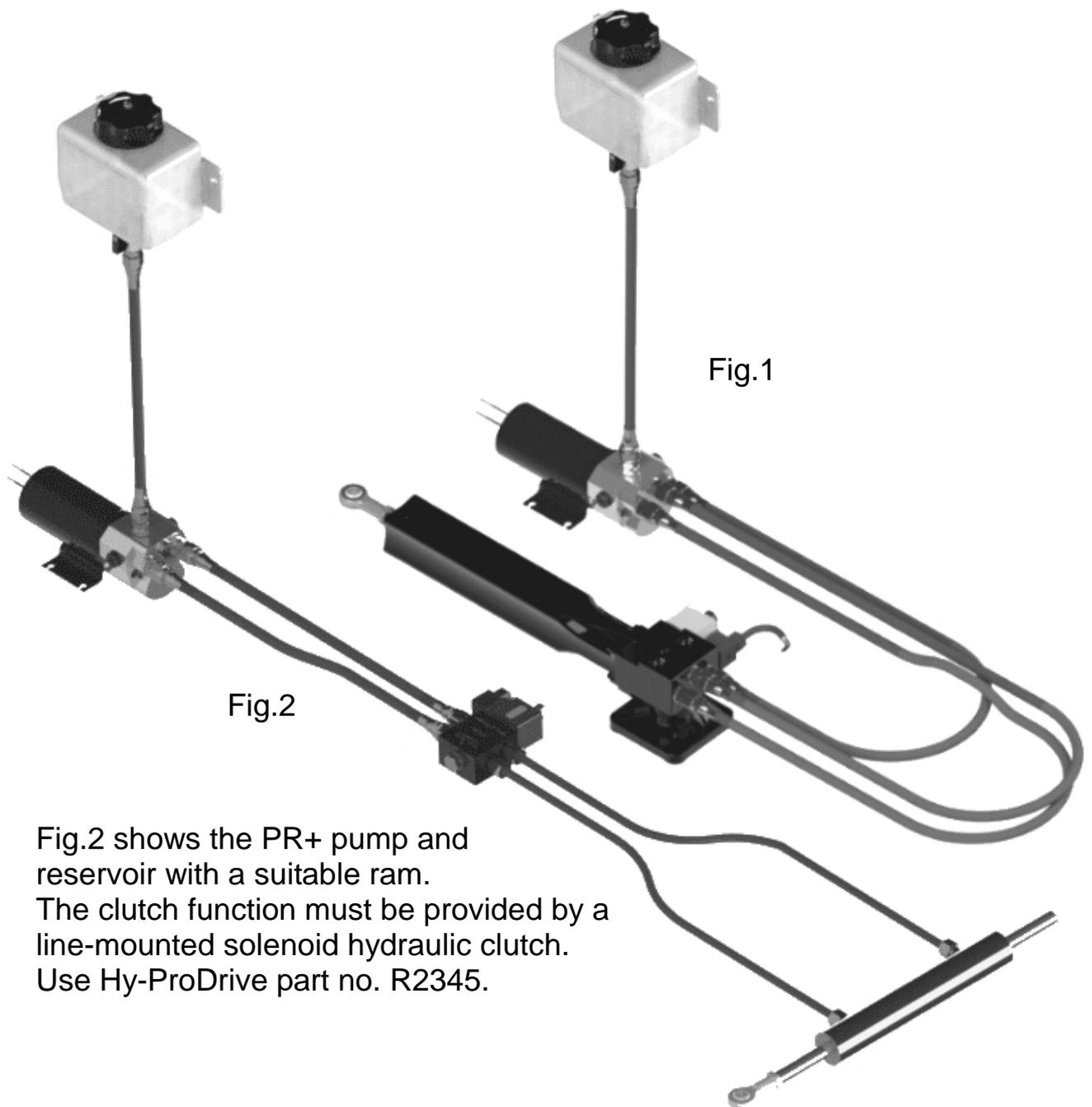
Fig.2 shows the PR+ pump and reservoir with a suitable ram. The clutch function must be provided by a line-mounted solenoid hydraulic clutch. Use Hy-ProDrive part no. R2345.
