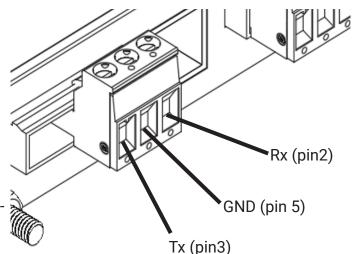
N.B Wire colours may vary between 3rd party cables/adapters (Pin numbers refer to a standard DB9 connector)
