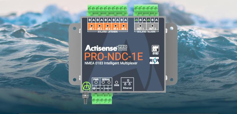
The PRO-NDC-1E is a RINA type-approved intelligent NMEA multiplexer, housed in a rugged stainless steel enclosure which provides isolation on all inputs and outputs.
