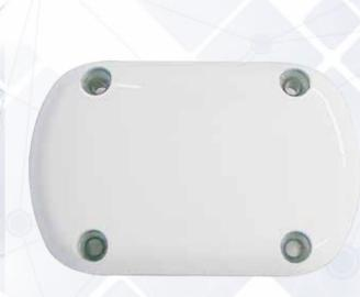
The RST703 dual mode patch antenna is supplied complete with bulkhead mount that enables it to be securely mounted without the connectors being exposed to the environment. The Beam RST703 dual mode patch antenna is fitted with an SMA female connector for GPS and a TNC for Iridium and will work with all Beam tracking products or other Iridium/GPS based devices.
