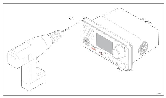
1. Using a drill and a 4 mm (5/32) drill bit, drill out the 4 mounting holes.
