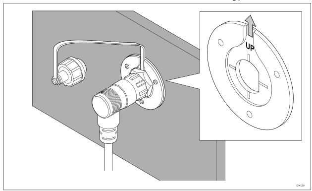
To ensure that the handset's connector points down when connected, orientate the mounting plate so that the lanyard grove is pointing straight up.
