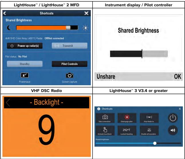
Multiple brightness groups can be configured. For example, these groups could be used to reflect the physical location of products on your vessel e.g.: helm and flybridge.
