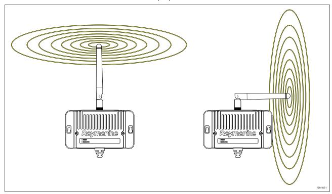
Keeping the antenna vertical should provide the best coverage for devices on the same plane as your hub. Positioning the antenna horizontally will provide better coverage above and below the hub.
