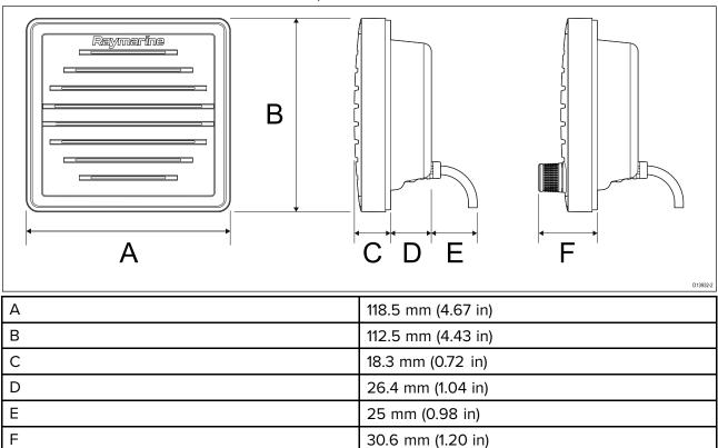
The Passive speaker includes a fitted 2 m (6.56 ft) audio cable terminated with a male RCA plug. The Active speaker includes a fitted 2 m (6.56 ft) power cable terminated with a spade connectors.
