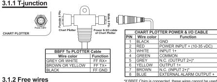
\*If BBFF Chirp is connected, these wires cannot be used
