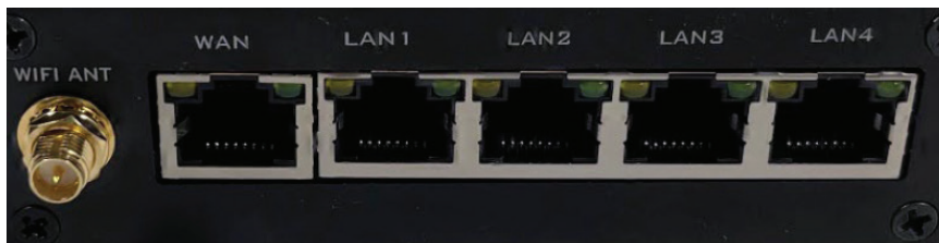
Figure 5.4.b - Wi-Fi antenna connector / WAN Port / LAN Ports 1, 2, 3, 4
