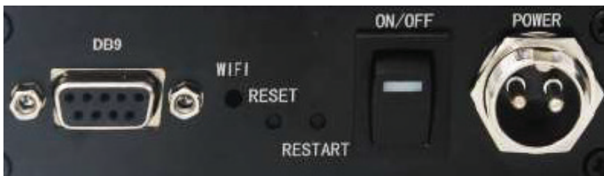
Figure 5.4.a - DB9 Serial Port / WiFi Indicator / Reset Button / Restart Button / On/Off / PWR Connector
