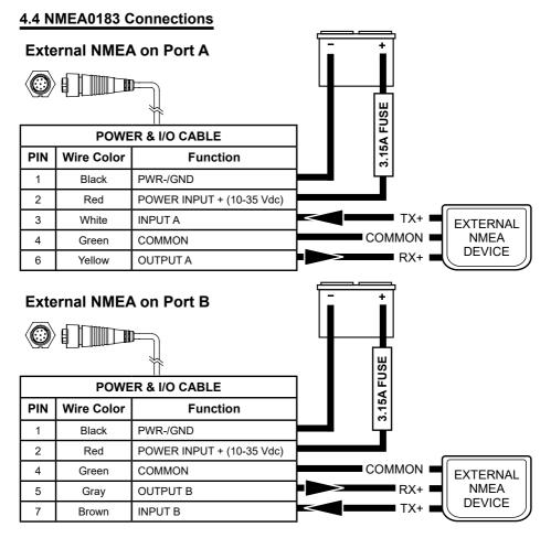
**Note:** NMEA-0183 input baud rate is automatically detected and selected. If you need to set the baud rate manually please go into the settings menu.
