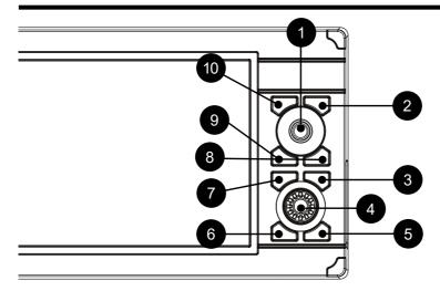
The joystick can move the cursor around the map or through menu items. Press [UP], [DOWN], [LEFT] or [RIGHT].
